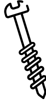
2½" or Longer Self Tapping Washer Head Cabinet Screws for joining cabinets to wall
