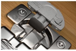
The development of the **TEC Soft-close** is based on the ever popular 3-dimensional TEC face frame hinge with a variety of overlays offered. The Soft-close mechanism is pre-mounted in to the interior of the hinge cup, therefore, no additional installation of the Soft-close is required. The drilling depth of the cup remains at 11mm and there are no protruding parts in the interior of the cabinet. Made in the USA, the **TEC Soft-close** offers quiet and effortless closing action every time.
